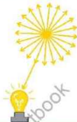
Fig. 8.2: An unpolarized light, due to incandescent bulb, has vibrations in all planes.
