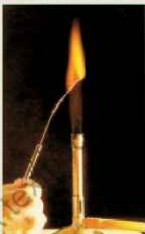
Monochromatic Light Sodium chloride in a flame gives out pure yellow light. This light is not a mixture of red and green.
